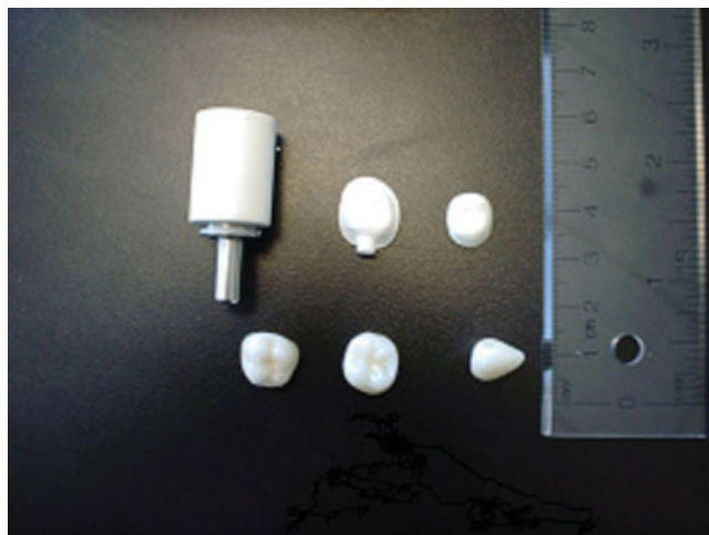
Figure 1. From left to right starting from the top: composite ingot, composite coping, densified coping, and three false teeth ready to be implanted into the mouth.
